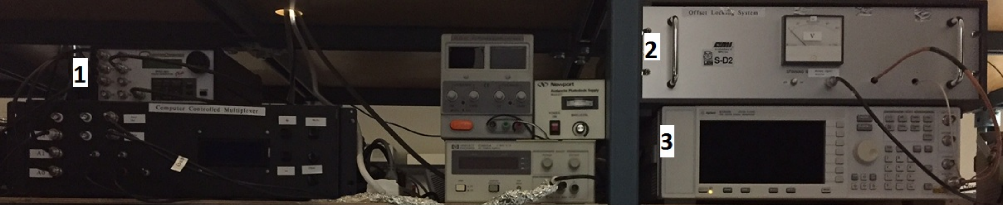
1. Arbitrary pulse generator, 2. Offset locking electronics, 3. rf signal generator
